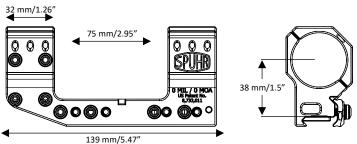
The mounts are machined from billet 7000 series aluminum and all aluminum parts are hardcoat anodized. The hardened steel side clamps feature Cerakote coating, and the Torx 20 ring and clamping screws are zinc-nickel coated for corrosion resistance and come pre-waxed from the factory to ensure proper torque values.
