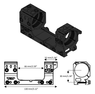
The mounts are machined from billet 7000 series aluminum and all aluminum parts are hardcoat anodized. The Torx 20 ring and clamping screws are zinc-nickel coated for corrosion resistance and come pre-waxed from the factory to ensure proper torque values.
