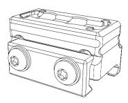
The SM-series of red dot sight mounts was designed to be the most rugged mounts possible. The mount consists of a mount body, a rail clamp, a set of clamping screws with washers, and five UC6S No 4 UNF x 6 screws for attaching the MRO to the mount.
