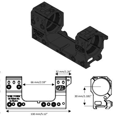
The mounts are machined from billet 7000 series aluminum and all aluminum parts are hardcoat anodized. The Torx 20 ring and clamping screws are zinc-nickel coated for corrosion resistance and come pre-waxed from the factory to ensure proper torque values.
