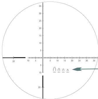
The R/T reticle uses a system that is based on a silhouette for quick ranging.
