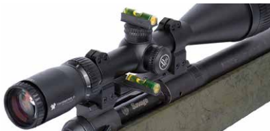
Use of bubble levels to square the riflescope (and reticle) to the base.
