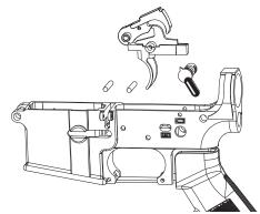
2a) Slightly loosen the grip on your lower receiver so the safety detent no longer engages the safety selector. Carefully, remove the safety selector. Some lowers may require you to fully remove the grip to do this.
