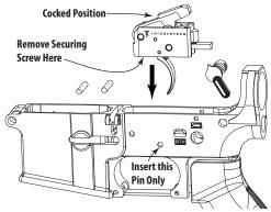
**CAUTION:** Be careful when removing the plastic securing screw as the trigger can rapidly release. Support the hammer and housing at all times.
